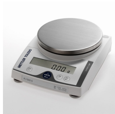
Figure 7 – Analytical scale ( \pm 0.01 g) used to assess boards water uptake by difference to the initial test sample weight.
