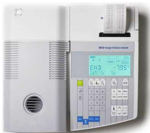
Figure 8 – Moisture analyzer used to assess solids content in each emulsion.
